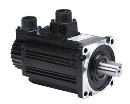
SureServo2 low inertia AC brushless servo motor, 1 kW, 3-phase input, 24-bit (16777216 ppr) encoder, integrated brake. For use with SureServo2 SV2A-4150 1.5 kW drive.
