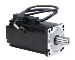
SureServo2 low inertia AC brushless servo motor, 750W, 3-phase input, 24-bit (16777216 ppr) encoder, integrated brake. For use with SureServo2 SV2A-4075 750W drive.
