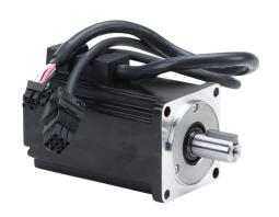
SureServo2 low inertia AC brushless servo motor, 400W, 3-phase input, 24-bit (16777216 ppr) encoder. For use with SureServo2 SV2A-4040 400W drive.
