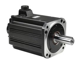
SureServo2 high inertia AC brushless servo motor, 11 kW, 3-phase input, 24-bit (16777216 ppr) encoder. For use with SureServo2 SV2A-4F00 15 kW drive.
