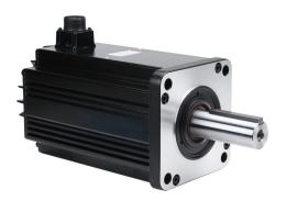
SureServo2 high inertia AC brushless servo motor, 7.5 kW, 3-phase input, 24-bit (16777216 ppr) encoder. For use with SureServo2 SV2A-4750 7.5 kW drive.
