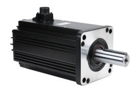
SureServo2 high inertia AC brushless servo motor, 7.5 kW, 3-phase input, 24-bit (16777216 ppr) encoder, integrated brake. For use with SureServo2 SV2A-4750 7.5 kW drive.
