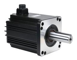
SureServo2 high inertia AC brushless servo motor, 5.5 kW, 3-phase input, 24-bit (16777216 ppr) encoder. For use with SureServo2 SV2A-4550 5.5 kW drive.
