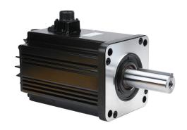
SureServo2 high inertia AC brushless servo motor, 5.5 kW, 3-phase input, 24-bit (16777216 ppr) encoder, integrated brake. For use with SureServo2 SV2A-4550 5.5 kW drive.
