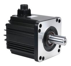
SureServo2 high inertia AC brushless servo motor, 4.5 kW, 3-phase input, 24-bit (16777216 ppr) encoder. For use with SureServo2 SV2A-4550 5.5 kW drive.
