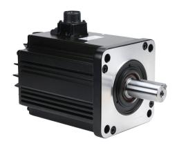
SureServo2 high inertia AC brushless servo motor, 4.5 kW, 3-phase input, 24-bit (16777216 ppr) encoder, integrated brake. For use with SureServo2 SV2A-4550 5.5 kW drive.
