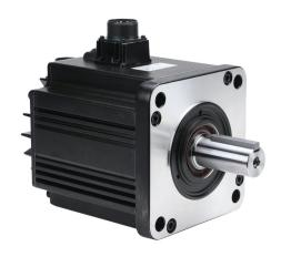
SureServo2 high inertia AC brushless servo motor, 3 kW, 3-phase input, 24-bit (16777216 ppr) encoder, integrated brake. For use with SureServo2 SV2A-4300 3 kW drive.
