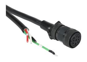
SureServo2 power flex cable, mating connectors, 65.6ft/20m cable length. For use with 230 VAC 2 kW and 3 kW and 460 VAC 3 kW SureServo2 motors without brake.
