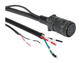
SureServo2 power cable, mating connectors, 32.8ft/10m cable length. For use with 230 VAC 2 kW and 3 kW and 460 VAC 3 kW SureServo2 motors with brake.
