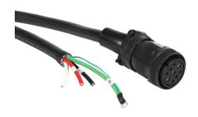
SureServo2 power flex cable, mating connectors, 32.8ft/10m cable length. For use with 230 VAC 2 kW and 3 kW and 460 VAC 3 kW SureServo2 motors without brake.
