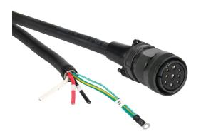
SureServo2 power cable, mating connectors, 16.4ft/5m cable length. For use with 230 VAC 2 kW and 3 kW and 460 VAC 3 kW SureServo2 motors without brake.
