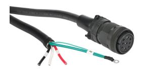
SureServo2 power cable, mating connectors, 9.8ft/3m cable length. For use with 230 VAC 2 kW and 3 kW and 460 VAC 3 kW SureServo2 motors without brake.
