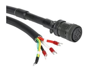
SureServo2 power flex cable, mating connectors, 9.8ft/3m cable length. For use with 230 VAC 4.5 kW and 460 VAC 4.5 kW-7.5 kW SureServo2 motors without brake.
