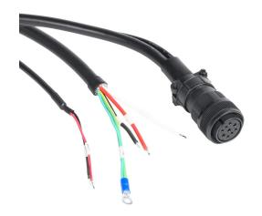
SureServo2 power cable, mating connectors, 65.6ft/20m cable length. For use with 230 VAC 1 kW low inertia and 460 VAC 1 kW-2 kW SureServo2 motors with brake.
