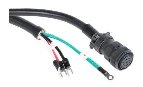
SureServo2 power cable, mating connectors, 65.6ft/20m cable length. For use with 230 VAC 1 kW medium inertia and 1.5 kW SureServo2 motors without brake.
