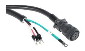
SureServo2 power cable, mating connectors, 9.8ft/3m cable length. For use with 230 VAC 1 kW medium inertia and 1.5 kW SureServo2 motors without brake.
