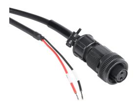
SureServo2 brake flex cable, mating connectors, 65.6ft/20m cable length. For use with 230 VAC 5.5 kW-15 kW and 460 VAC 11 kW and 15 kW SureServo2 motors with brake.
