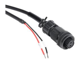
SureServo2 brake flex cable, mating connectors, 32.8ft/10m cable length. For use with 230 VAC 5.5 kW-15 kW and 460 VAC 11 kW and 15 kW SureServo2 motors with brake.
