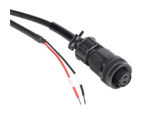
SureServo2 brake flex cable, mating connectors, 9.8ft/3m cable length. For use with 230 VAC 5.5 kW-15 kW and 460 VAC 11 kW and 15 kW SureServo2 motors with brake.
