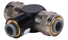
NITRA pneumatic threaded fitting, shuttle valve, anodized aluminum body, nickel-plated brass threads, (3) 1/4in push-to-connect.
