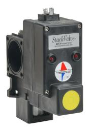
CITO StackValve modular solenoid valve, 2-way, 2-position, N.C., glass-filled nylon body, stackable, Cv=8.5, 120 VAC operating voltage, 12VA, 18mm DIN style wiring plug. RA-3903 high-flow turbine and SF-9130 screen included.
