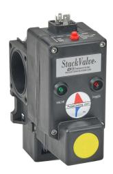
CITO StackValve modular solenoid valve, 2-way, 2-position, N.C., glass-filled nylon body, stackable, Cv=8.5, 24 VAC/VDC operating voltage, 7.2W, 18mm DIN style wiring plug. RA-3903 high-flow turbine and SF-9130 screen included.
