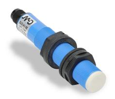
Micro Detectors ultrasonic proximity sensor, tubular, 18mm diameter x 90mm body, polybutylene terephthalate housing, 0-10 VDC analog output, 200-1500mm sensing distance, IP67, 4-pin M12 quick-disconnect.
