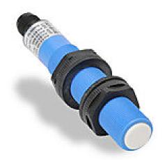
Micro Detectors ultrasonic proximity sensor, tubular, 18mm diameter x 90mm body, polybutylene terephthalate housing, 0-10 VDC analog output, 100-600mm sensing distance, IP67, 4-pin M12 quick-disconnect.
