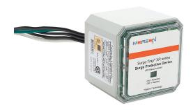
Mersen STXR series power Surge Protective Device (SPD), 20 kA discharge current, 480/277 VAC 3-Phase Wye, neutral ground protection, parallel circuit, NEMA 4/4X enclosure rating, 3/4in NPSM mount.
