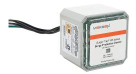
Mersen STXR series power Surge Protective Device (SPD), 10 kA discharge current, 480 VAC 3-Phase Delta, parallel circuit, NEMA 4/4X enclosure rating, 3/4in NPSM mount.
