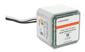
Mersen STXR series power Surge Protective Device (SPD), 20 kA discharge current, 240/120 VAC Split Phase, parallel circuit, NEMA 4/4X enclosure rating, 3/4in NPSM mount.
