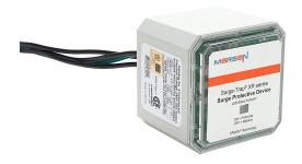
Mersen STXR series power Surge Protective Device (SPD), 20 kA discharge current, 240 VAC 3-Phase Delta, parallel circuit, NEMA 4/4X enclosure rating, 3/4in NPSM mount.
