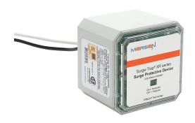
Mersen STXR series power Surge Protective Device (SPD), 20 kA discharge current, 120 VAC 1-Phase, parallel circuit, NEMA 4/4X enclosure rating, 3/4in NPSM mount.
