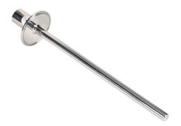
ProSense sanitary thermowell, 1/2in female NPT probe connection, 2in sanitary tri-clamp process connection, 316 stainless steel body, 12-1/4in overall length, 0.260in bore.
