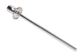
ProSense sanitary thermowell, 1/2in female NPT probe connection, 1-1/2in sanitary tri-clamp process connection, 316 stainless steel body, 12-1/4in overall length, 0.260in bore.
