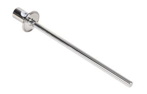
ProSense sanitary thermowell, 1/2in female NPT probe connection, 1-1/2in sanitary tri-clamp process connection, 316 stainless steel body, 12-1/4in overall length, 0.260in bore.
