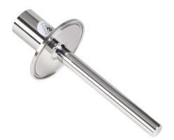
ProSense sanitary thermowell, 1/2in female NPT probe connection, 2in sanitary tri-clamp process connection, 316 stainless steel body, 6-1/4in overall length, 0.260in bore.
