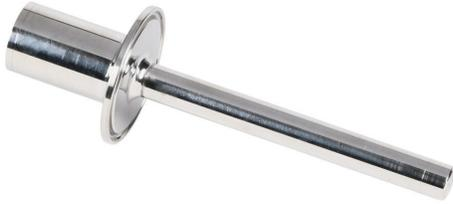
ProSense sanitary thermowell, 1/2in female NPT probe connection, 1-1/2in sanitary tri-clamp process connection, 316 stainless steel body, 6-1/4in overall length, 0.260in bore.
