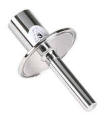
ProSense sanitary thermowell, 1/2in female NPT probe connection, 2in sanitary tri-clamp process connection, 316 stainless steel body, 4-1/4in overall length, 0.260in bore.
