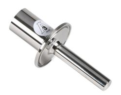
ProSense sanitary thermowell, 1/2in female NPT probe connection, 1-1/2in sanitary tri-clamp process connection, 316 stainless steel body, 4-1/4in overall length, 0.260in bore.
