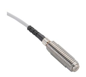
Metrol limit switch, stopper bolt, 10mm diameter, threaded, 1.5mm pitch, 38.2mm length, 4.5mm flat head, stainless steel, 1.5mm plunger, 2N contact force, (1) N.O. contact(s), 6.5ft/2m cable length, pigtail.
