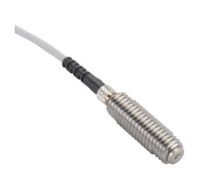
Metrol limit switch, stopper bolt, 10mm diameter, threaded, 1.5mm pitch, 38.2mm length, 4.5mm flat head, stainless steel, 1.5mm plunger, 2N contact force, N.O. contact(s), 6.5ft/2m cable length, pigtail.
