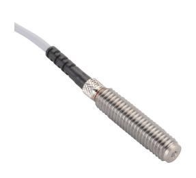
Metrol limit switch, stopper bolt, 8mm diameter, threaded, 1.25mm pitch, 38.2mm length, 4.5mm flat head, stainless steel, 1.5mm plunger, 2N contact force, (1) N.O. contact(s), 6.5ft/2m cable length, pigtail.
