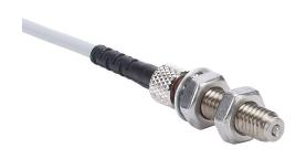
Metrol limit switch, stopper bolt, 6mm diameter, threaded, 1mm pitch, 31.7mm length, 3.4mm flat head, stainless steel, 1.5mm plunger, 2N contact force, (1) N.O. contact(s), 6.5ft/2m cable length, pigtail.
