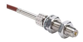
Metrol limit switch, high temperature, stopper bolt, 6mm diameter, threaded, 1mm pitch, 31.7mm length, 3.4mm flat head, stainless steel, 1.5mm plunger, 1N contact force, N.O. contact(s), 6.5ft/2m cable length, pigtail.
