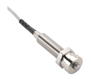
Metrol limit switch, stopper bolt, 10mm diameter, threaded, 1.5mm pitch, 55.4mm length, 5mm radius head, stainless steel, 5.5mm plunger with upward cover, 4N contact force, (1) N.O. contact(s), 6.5ft/2m cable length, pigtail.
