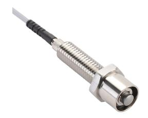
Metrol limit switch, stopper bolt, 10mm diameter, threaded, 1.5mm pitch, 55.4mm length, 5mm radius head, stainless steel, 5.5mm plunger with downward cover, 4N contact force, (1) N.O. contact(s), 6.5ft/2m cable length, pigtail.
