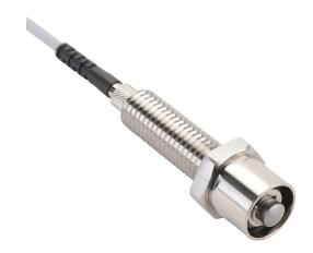
Metrol limit switch, stopper bolt, 10mm diameter, threaded, 1.5mm pitch, 55.4mm length, 5mm radius head, stainless steel, 5.5mm plunger with downward cover, 4N contact force, N.O. contact(s), 6.5ft/2m cable length, pigtail.
