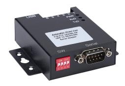
SureStep PC adapter, USB B to RS-485. For use with SureStep STP-MTRD-xxxxxR integrated stepper motor/drives. (1) 3ft USB A to USB B cable included. Requires STP-485DB9-CBL-2 communication cable.
