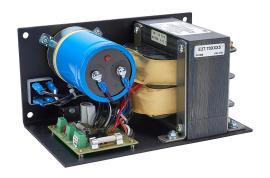
SureStep unregulated linear power supply, 70 VDC @ 5A/350W and 5 VDC @ 0.5A/2.5W, 120/240 VAC nominal input, 1-phase, open frame, aluminum housing, chassis mount, screw terminals.
