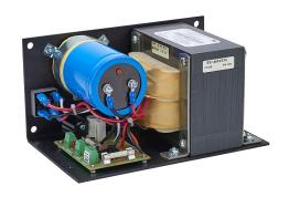
SureStep unregulated linear power supply, 48 VDC @ 10A/480W and 5 VDC @ 0.5A/2.5W, 120/240 VAC nominal input, 1-phase, open frame, aluminum housing, chassis mount, screw terminals.
