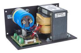
SureStep unregulated linear power supply, 48 VDC @ 5A/240W and 5 VDC @ 0.5A/2.5W, 120/240 VAC nominal input, 1-phase, open frame, aluminum housing, chassis mount, screw terminals.
