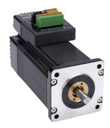
SureStep DC integrated stepper motor/drive, advanced microstepping, NEMA 24 frame, IP20, 6A, 12-70 VDC, bipolar, 340 oz-in holding torque, 1.8-degree step angle, 200 to 51200 steps per revolution, (1) RS-485 (4-pin) port(s).
